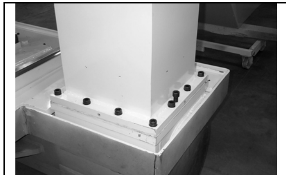
Figure 3.6 STG bridge - base joint
