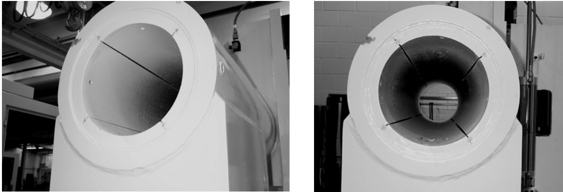
Figure 4.8 ShearDamper™ based on split tube design in Star Cutter STG 5-axis grinder
