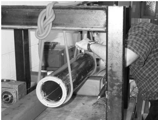
Figure 5.9 Free-free beam setup (a) and 16 measuring points
