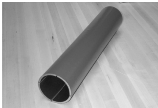
Figure 5.1 Split tube constraining layer, raw tube (a) and wrapped with ISODAMP TM C-1002 (b)
